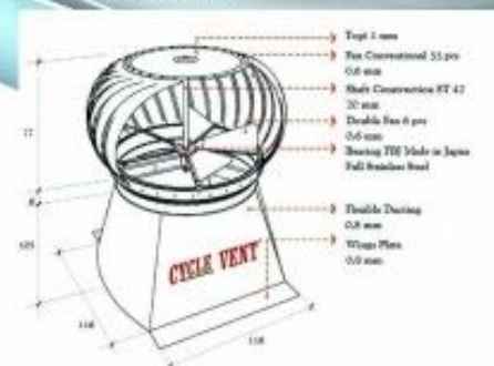
CYCLEVENT TURBINE VENTILATOR NON ELECTRIC TYPE CV-105 Bahan : Aluminium & Stainless Steel 430/304 Bearing : SKF Full Stainless Steel, Made In Japan Diameter : 105 CM = 42" Dimensi : 347 x 154 x 154" Berat : 20.5 kg / 25 kg Kapasitas Hisap : 5940 M 3 / menit
