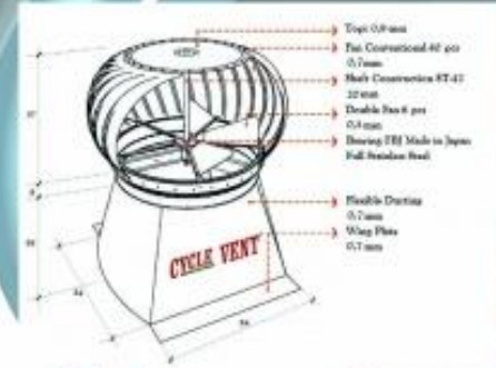
CYCLEVENT TURBINE VENTILATOR NON ELECTRIC TYPE CV-75 (2) Bahan : Aluminium & Stainless Steel 430/304 Bearing : SKF Full Stainless Steel, Made In Japan Diameter : 75 CM = 30" Dimensi : 226 x 100 x 100" Berat : 13.5 kg / 19.5 kg Kapasitas Hisap : 3035 M 3 / menit
