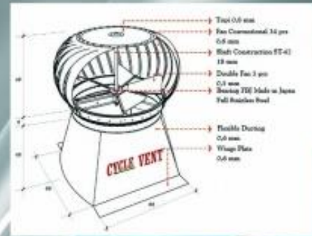
CYCLEVENT TURBINE VENTILATOR NON ELECTRIC TYPE CV-60(2) Bahan : Aluminium & Stainless Steel 430/304 Bearing : SKF Full Stainless Steel, Made In Japan Diameter : 60 CM = 24" Dimensi : 198 x 86 x 36" Berat : 8.5 kg / 18.5 kg Kapasitas Hisap : 1940 M 3 / menit
