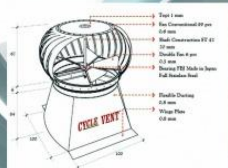
CYCLEVENT TURBINE VENTILATOR NON ELECTRIC TYPE CV-90 Bahan : Aluminium & Stainless Steel 430/304 Bearing : SKF Full Stainless Steel, Made In Japan Diameter : 90 CM = 36" Dimensi : 267 x 137 x 137" Berat : 19.5 kg Kapasitas Hisap : 4370 M 3 / menit
